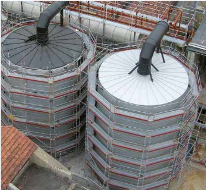
Air purification system, Spain. Material: HD-PE
