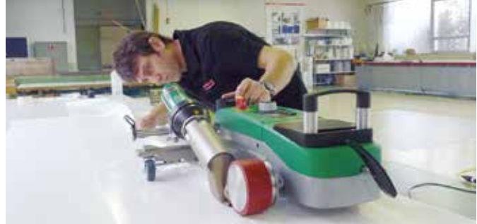
Very easy hem and piping welds with the hem / piping welding kit.
