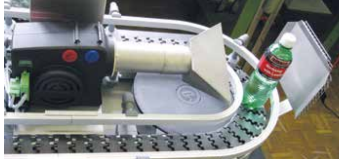
HOTWIND SYSTEM with wide slot nozzle integrated in a blow-off application.
