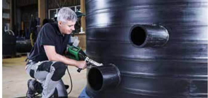
The powerful WELDPLAST S4 in use.
